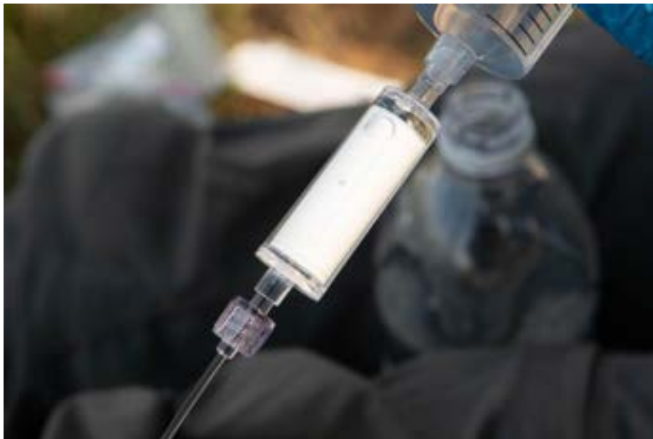
Figure 33. Filtering water through a Sterivex filter for eDNA collection.
