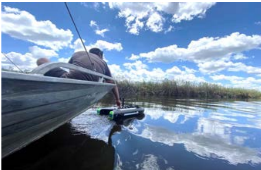
Figure 38. The ADCP deployed on the Cuando River.
