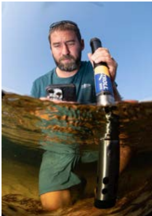
Figure 27. In Situ Aqua Troll 600 multi-parameter sonde.
