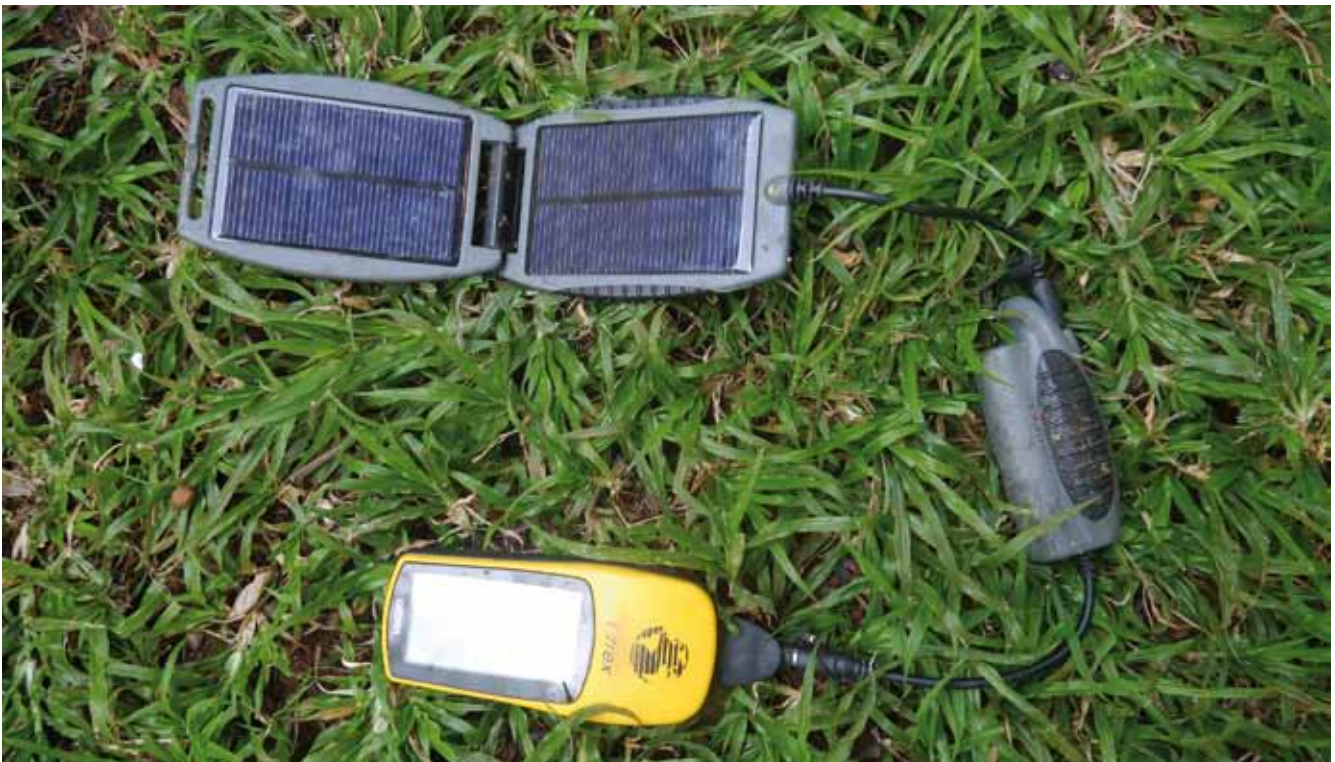
Solar panels and chargers can be used to recharge GPS devices, VHF radios and other equipment. © CDC
